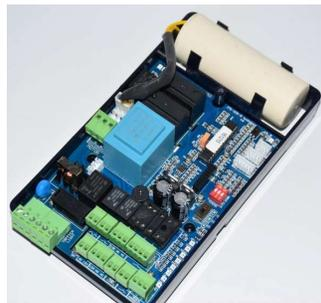
**Gambar 7.** *Mainboard* Atau *Mikrokontroler*
