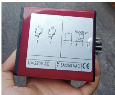
**Gambar 10.** *Vehicle Loop Detector (VLD)*
